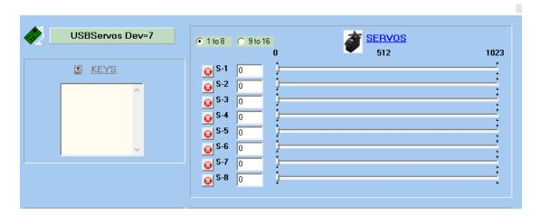
My servo is "S-1". By moving the slider for "S-1", I can see the position-value changing when I move the slider (the value is 0 in the screenshot above).
