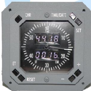
This particular module has an additional option for us to know at all times if we are in CHR or ET mode: if mode ET only blink dot point what separate the minutes and seconds of the lower display and when we remain in CHR mode, the righter dot point of the bottom display (which is stamped with text "CHR") will remain on.
