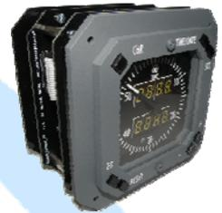
The module is fully configurable with SIOC, making it compatible with FSX and any add-ons you have installed, if you use the correct script. On the website of Opencockpits is available a generic script that works with all basic FSX planes though options can be added to integrate into specific performance of any add-on.
