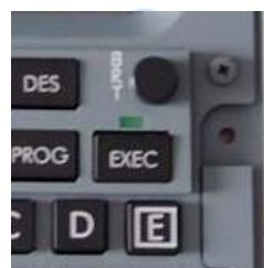
Simply turn the brightness button to go from zero to full brightness and vice versa
