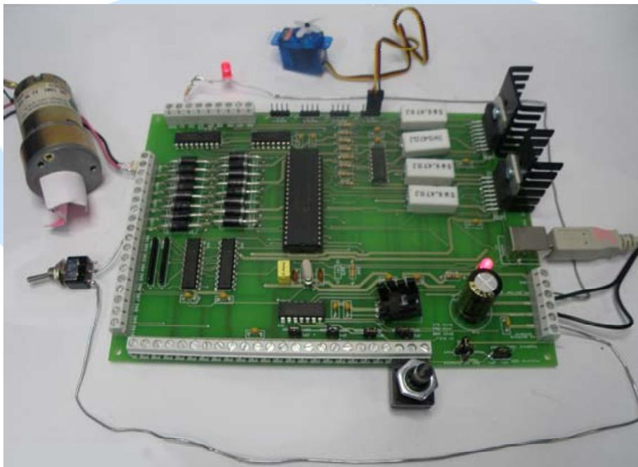
Our test engine and servo operate at 5V, so we will feed 5V to the USB-DCMotors Plus card from an external power supply for the tests, i.e. closed JP1 in POS2 and JP6 in POS3. The motor will be connected to MOT-1 pins 1 and 2 output (the direction of rotation can be changed either via SIOC, either via hardware changing the connection of the motor cables). The potentiometer is connected to input AN1 (J6 with open JP2), the led to the output O1 and to the
