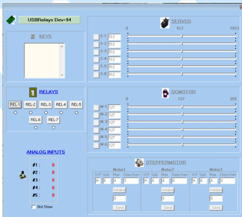
How we can see the analog input #1 shows the potentiometer value and the rest are at 0, if we turns the potentiometer we will see the value changing to more or less or vice versa (it depends of wire connection), we can change the turn direction changing the J3 wires to opposite pins or using a SIOC script.
